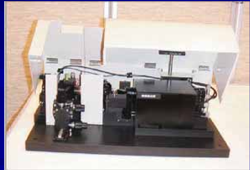
3-D microscope tomographic measurement system prototyped
