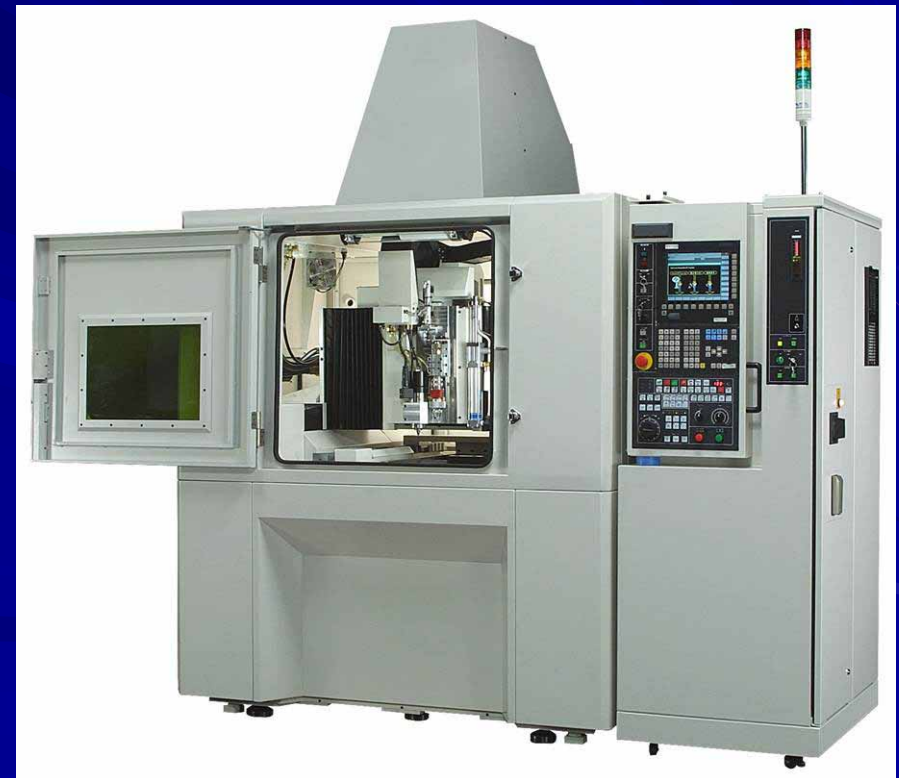
Laser metal modeling hybrid machining unit
