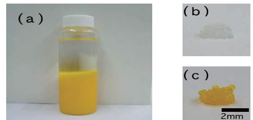
Fig. (a) thermo-sensitive adsorbents: (b) before fixed (c) after fixed
