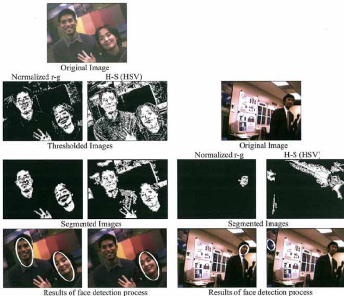
Figure 6. Examples of the detection of skin pixels and of the faces of Asian subjects in complex scene images, for the normalized r-g chrominance space (left column) and for the H-S space (HSV color space) (right column), by use of the single Gaussian chrominance model. The original images were recorded with the SGI camera (see Subsection 5 of Phase I Section for a detailed overview of the face detection algorithm).
