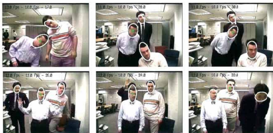
Figure 25. Simultaneous detection of the faces of two Caucasian subjects and of one Asian subject.
