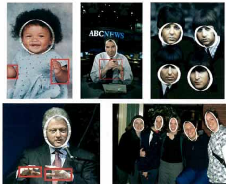
Figure 22. Examples of the successful detection of faces and of hands of Caucasian subjects in images selected from various sources, mostly from the World Wide Web.
