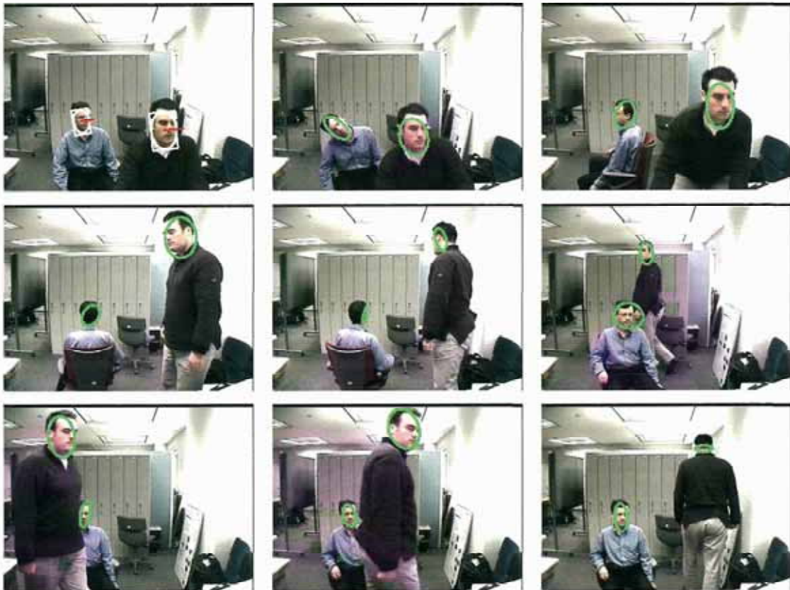
Figure 28. Simultaneous tracking of the faces of two Caucasian subjects (without camera control).
