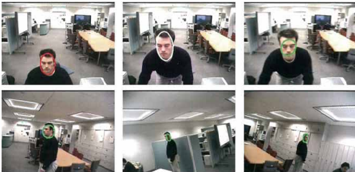
Figure 27. Successive SVM-based detection, skin color-based detection, and camera-controlled tracking of the face of a Caucasian subject (active zoom is not performed here).
