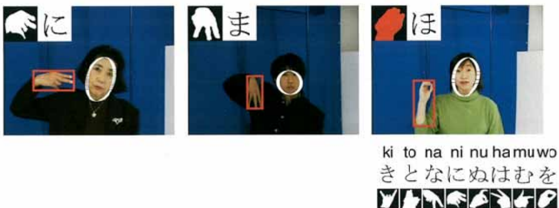
Figure 20. Example of the recognition of three different hand postures representing the phonemes “ni”, “ma” and “wo” respectively. In the rightmost image, the posture for “wo” was misclassified as the posture for “ho”, because the forearm of the subject is exposed and connected to her hand.
