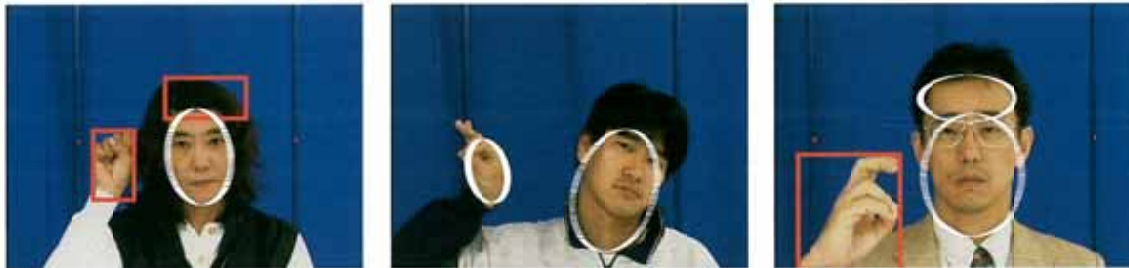
Figure 19. Example of problems occurring with the present face and hand detection system. From left to right: detection of a hair region as a hand, misclassification of a hand as a face, and double detection of a face due to the presence of glasses.
