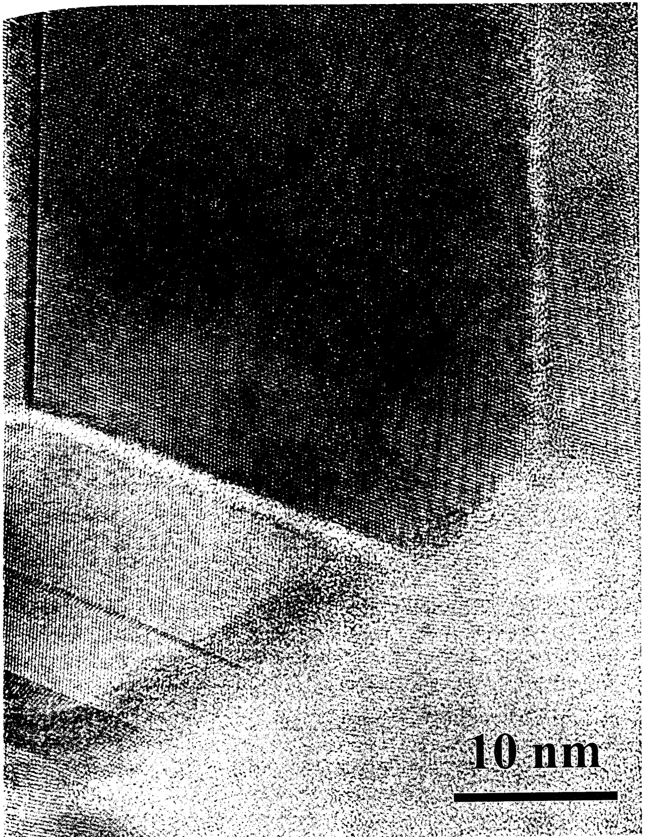
Fig. 1 HREM image of grain boundaries with amorphous films in a AYC SiC sample.
