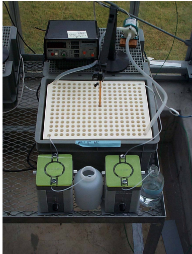
Fig. 3 Hydroponic system with pH controller and water circulator
