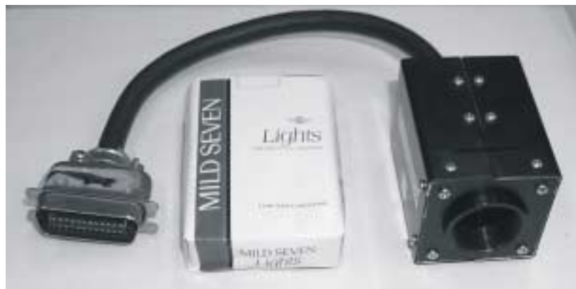
Fig. 2. Photograph of the camera unit. The size of the camera is similar to that of a package of cigarettes.
